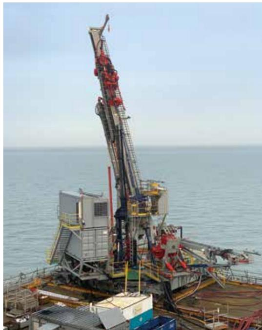
**Rig operating in SDD mode** on existing slanted well slot
