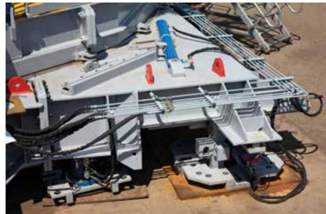
Stepping shoe of **XY skidding system** to skid along existing platform beams
