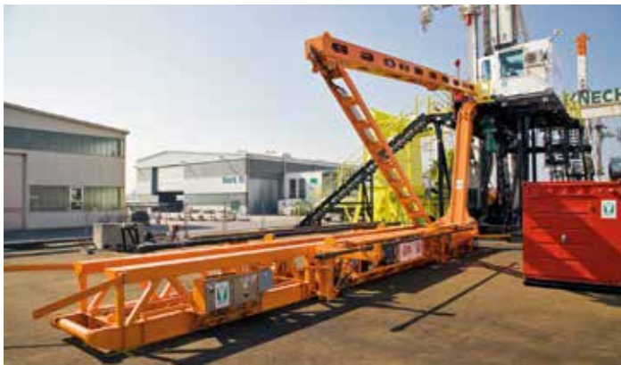
Hydraulic power catwalk for hands-off pipe handling
