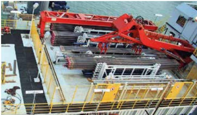
Automated pipe racking system on cantilever deck with gantry crane and pipe boxes (man free no-go area)
