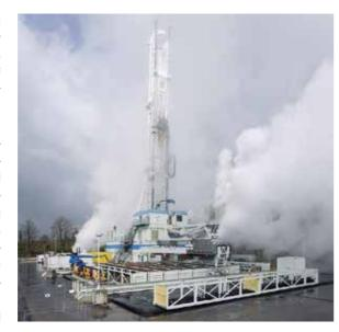
Lift tests after drilling show the productivity of the geothermal wells
