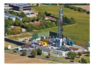
Silent box-on-box rig drilling in close proximity to built-up areas
