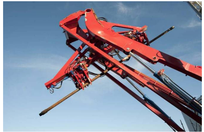
Hydraulic pipe handler with drill pipe.
